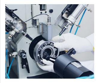
Once assembled, BW bearings are tested for noise and precision. Therefore, quality inspection is the necessary procedure before BW bearings leave manufacturing factories.
