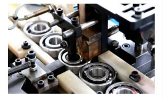
Assembly of the bearings is also carried out via automatic lines without the direct intervention of the operator. During and at the end of each production phase of BW bearings, the bearings are routinely inspected and conformity tested to ensure that they meet the strict quality control guidelines.
