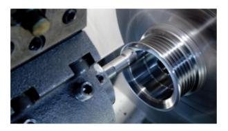
Create favorable conditions for the subsequent grinding process. Turning method: Concentrated process method: Complete small volume production of all turning operations on a single machine. Dispersion process method: A mass production of a certain turning process is completed on a single device.
