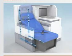
LM Guide Model SR are used in the seat sliding mechanism of small aircraft. Because the floors in aircraft are generally made from sheet metal, measuring errors relating to mounting sections are common, and mounting can be a lengthy process. Because Model SR have excellent error absorbing capabilities, they can be mounted directly on the floor of aircraft, reducing the work required for assembly
