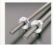
The Screw Nut is a sliding feed nut compatible with the standards for a 30-degree trapezoidal screw thread. Formed by die-casting special bearing alloy of superb abrasion resistance, it is an inexpensive high precision product.
