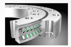
By integrating double-row small-diameter rollers on the raceway, the number of rollers incorporated in this new model (RW228) is approximately 5 times that of Cross-Roller Ring model RU. While maintaining the compactness, it achieves higher rigidity and accuracy and a lower torque. In addition, the inner and outer rings in integrated structures have mounting holes, allowing the product to be directly mounted to the machine.
